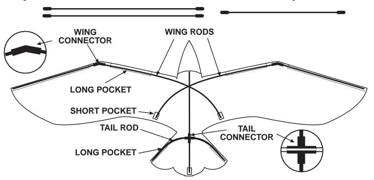
**STEP 1**: Insert one end of each wing rod through the long pocket and into the wing connector.
