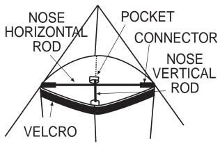
STEP 1: Open the velcro closure to expose the inside of the kite. Then insert the ends of the vertical rod into the pockets at the top and bottom. Then insert each end of the horizontal rod into the connectors at each side.
