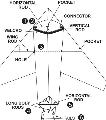
rod through the hole and into the pocket inside the body of the kite. Then insert the other end into the pocket in the tail. (NOTE: repeat this step for the right and left tails.)
