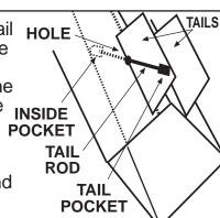
STEP 6: Insert the ends of the horizontal rod into the connectors on each side of the rear of the kite.
