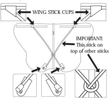
5. Insert the short kite stick into the top stick holder. Insert each end into each wing stick cup.
