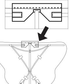
9. Peel the backing sheet off the narrow top part of the reinforcement sticker and fold over the top of kite to the other side and press firmly.
