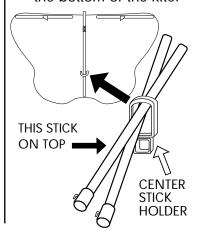
4. Spread the two longest sticks into a "X" shape. Insert the top of each stick into the wing stick cups. Insert the bottom of the sticks with the end caps into the holes in kite.
