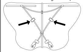
8. Place the top reinforcement sticker **UNDER** the top of the kite and align with sticks. The outlines of the kite sticks are printed on the sticker to guide you. After you understand where the sticker goes then peel the backing sheet off the **BOTTOM PART** of the reinforcement sticker. Place the sticker under kite as before and press the kite firmly to sticker. DO NOT PEEL OFF NARROW TOP PART OF THE
