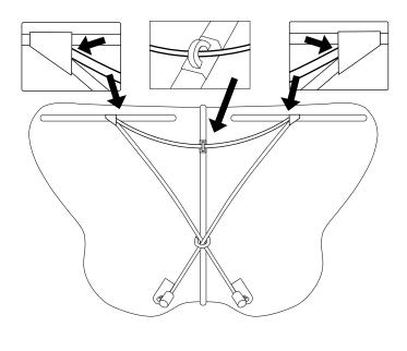
6. Place the top reinforcement sticker sheet on the kite and measure the distance from the end cap. Peel off one wing reinforcement sticker and place it over the stick on the kite at the end of the sheet. Press sticker down so the kite stick
